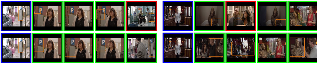
Figure 3.2: Sum/max comparison on TRECVID. Top 4 rankings and object locations obtained for queries 9098: a P (parking automat) sign and 9076: this monochrome bust of Queen Victoria from the INS 2013 dataset (query images surrounded in blue). Comparison between the rankings generated using RPA-sum (top) and RPA-max (bottom), after the filtering stage with IPA-sum. Regressed bounding box coordinates have been disabled for visualization.
