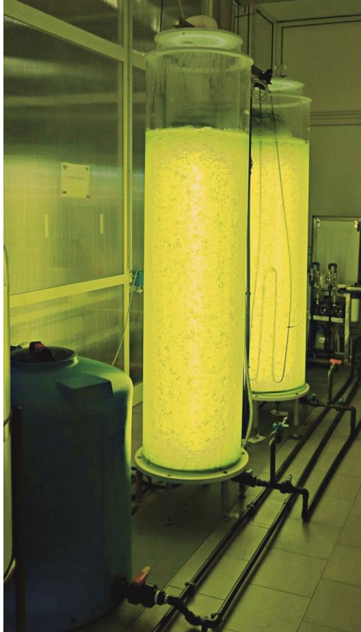
Figure 5.2: Column photobioreactors of 120 L with a temperature and aeration regulation control system. The system was monitored with a Programmable Logic Controller (PLC).
