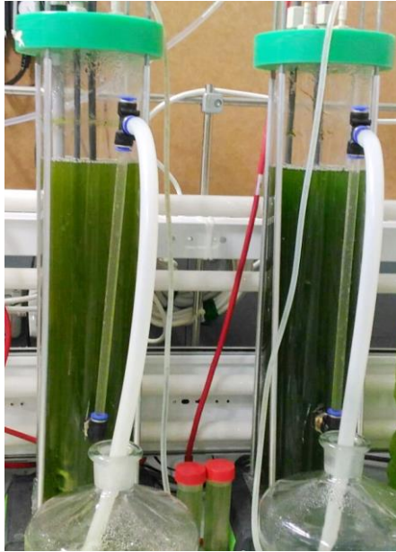
Figure 6.1: two column PBRs used for the experiment. This system is located in Politecnico di Milano, (Department of Civil and Environmental Engineering)
