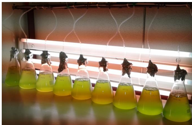
Figure 4.2: Pre-culture inocula in Erlenmeyer flasks in Pyrex glass enriched with Guillard F/2 medium (International Marine Centre - IMC Foundation)
