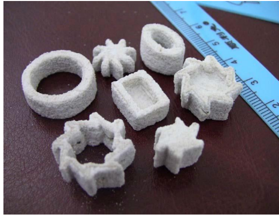
Figure 1.9 - Complex green parts created with indirect SLS by using one of the best laser parameters (Frequency: 10 kHz, Pulse width: 10 \mu s, laser power: 6 W, scan speed: 20 mm) [18]
