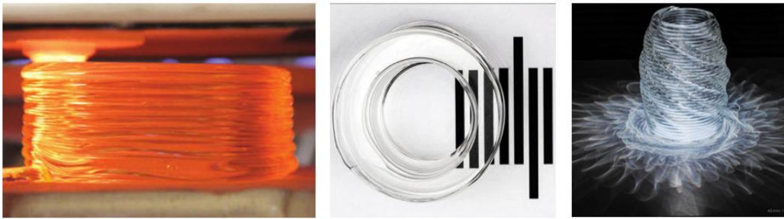
Figure 1.16 - Molten glass material 3D extrusion system (left), high object transparency (middle), and complex caustic patterns (right) [36]
