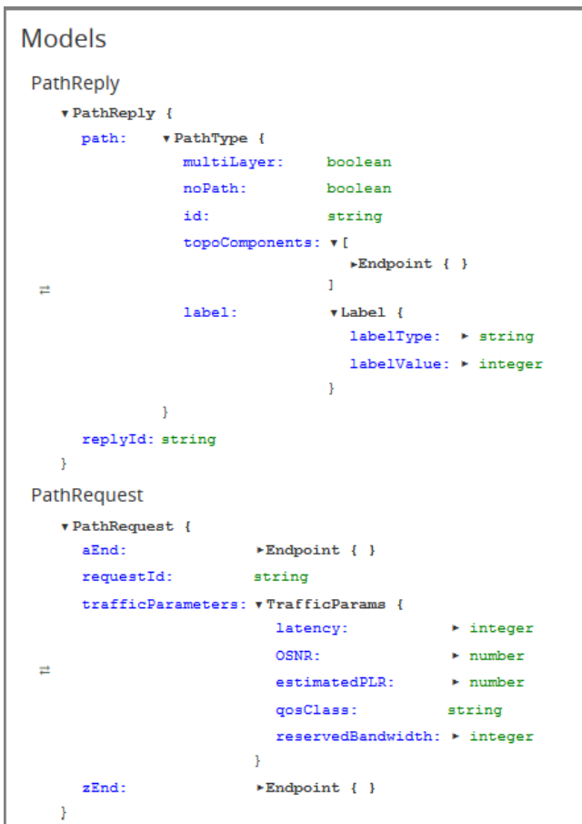
Figure A.10: COP Path Computation service JSON Data models SWAGGER editor display.
