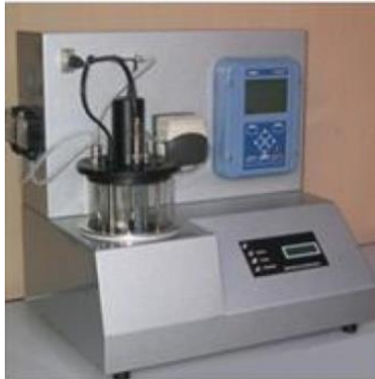
Figure 5.2 Image of the BMT respirometer model used for the respirometry tests (Source: Surcis.com)
