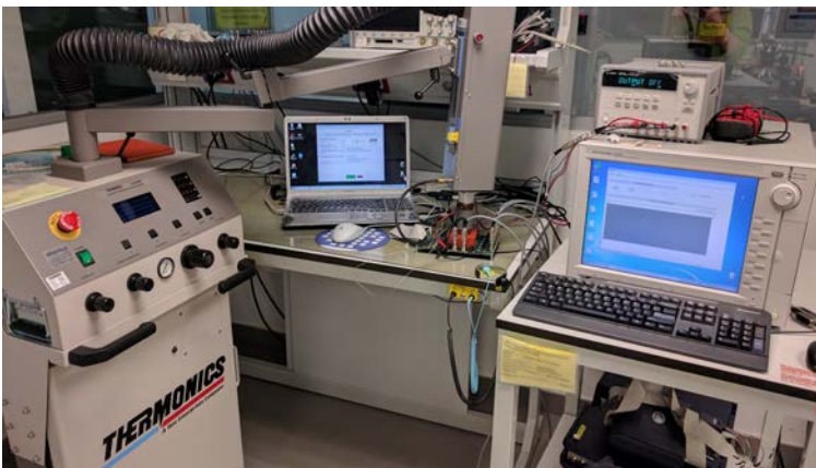
Figure 3.11: Laboratory characterization setup for variability testing corresponding with the schematic drawing shown in Figure 3.10.
