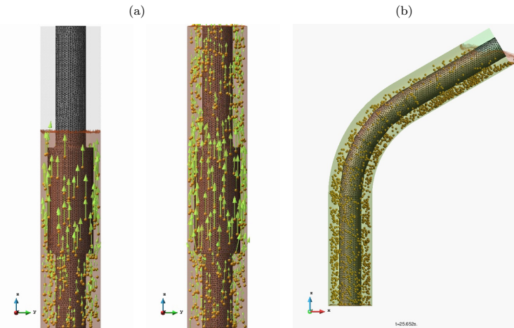
Fig. 9: Simulation of drill cuttings transported in straight and curved wellbores by mud as a result of a drilling operation. Arrows denote the velocity vector of each particle
