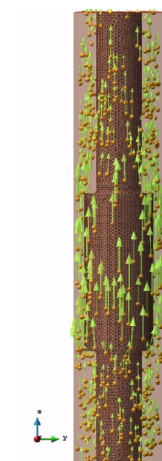
Figure 57: Particulate flow around a tooljoint in the drill string
