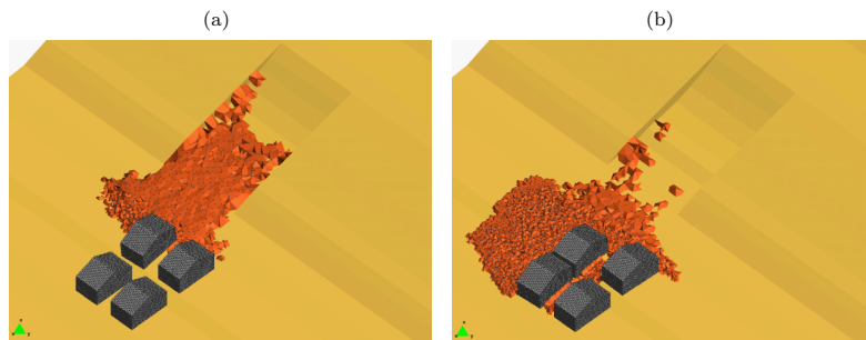
Fig. 16: 3D PFEM simulation of a landslide falling on four houses
