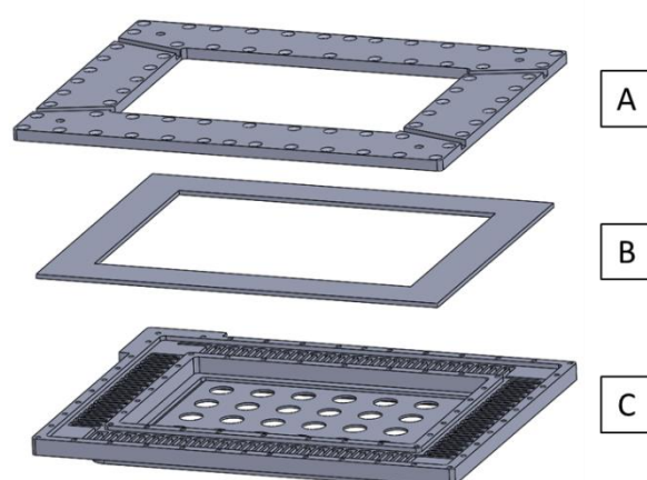
Figure 51, Explode view of the heat stage. Heat stage base(A), sealing rubber(B) and heat stage top(C).
