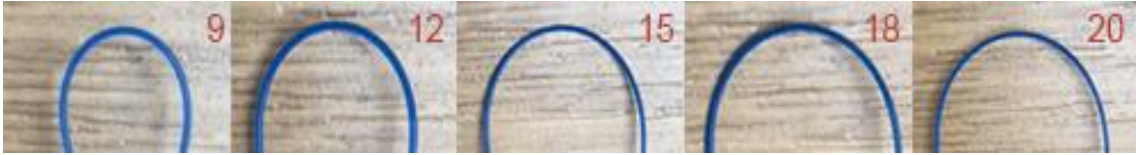
Figure 5. Laser fiber-bending diameters tested: 9, 12, 15, 18, and 20 mm.
