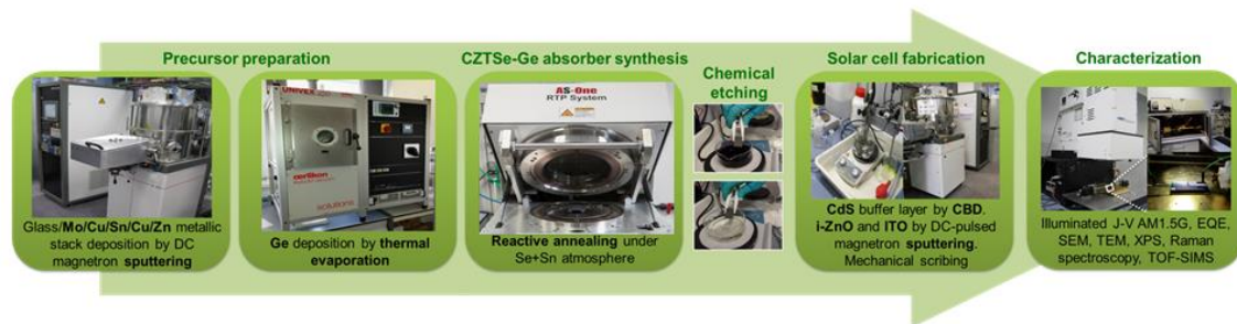
Figure 2.1 Schematics of the typical fabrication and characterization process for CZTSe solar cells by Rapid Thermal Processing at IREC.
