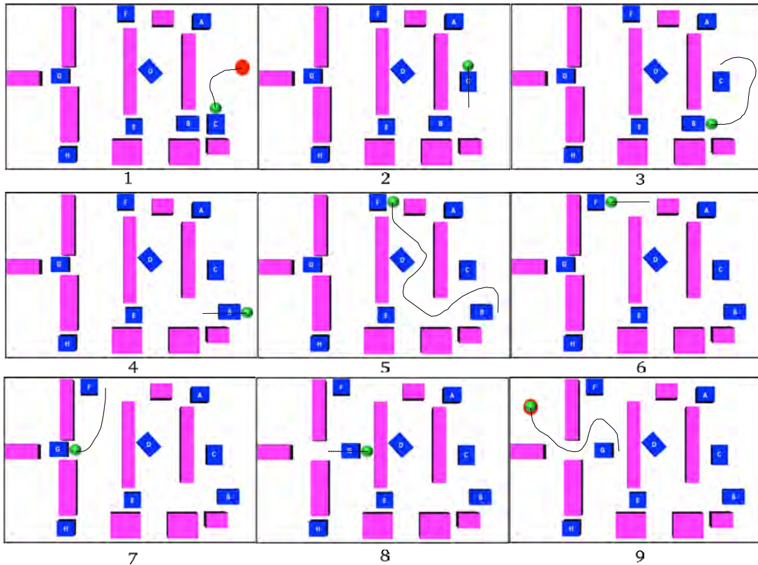
Figure 5.7: Snapshots of the task execution that involves the following actions: 1) transit to C, 2) pull C, 3) transit to B, 4) pull B, 5) transit to F, 6) push F, 7) transit to G, 8) pull G, 9) transit to Goal (The solution can be visualized in https://sir.upc.edu/projects/kautham/videos/manip.mp4 ).
