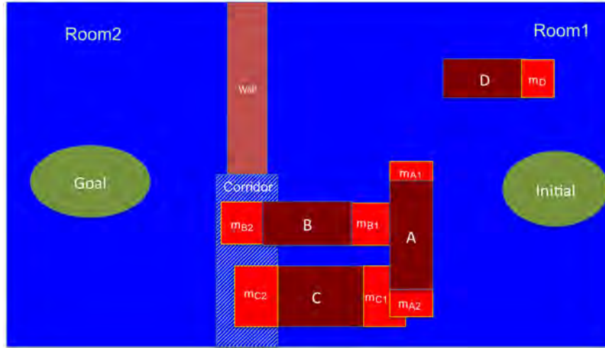
Figure 4.6: A NAMO manipulation problem where a robot must find a feasible path to reach the goal region avoiding the fixed wall. corridor is a connecting region to connect both rooms together.
