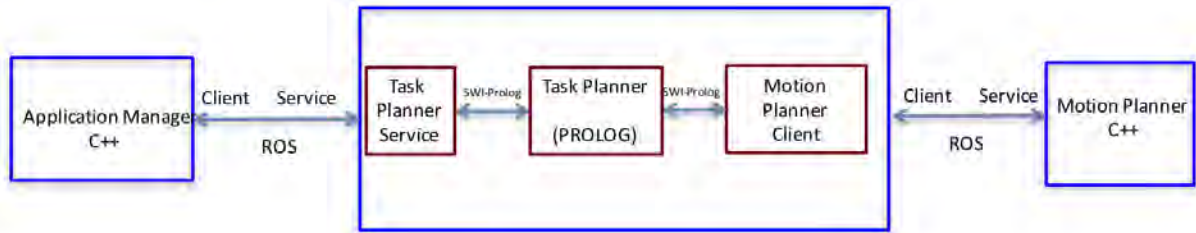
Figure 8.6: Prolog-based task planning as either service or client to communicate with motion planning.
