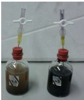
Figure 3.8. Example of slurries prepared to determine potential denitrification and DNRA activities in sediment of Empuriabrava FWS-CW.
