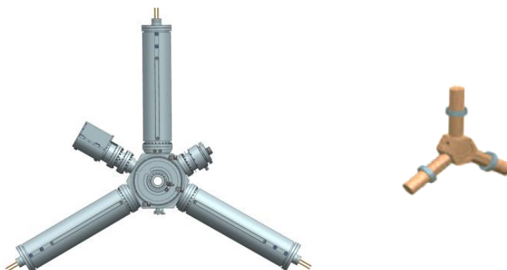
Figure 2-6: main RF cavity (left) vs. scaled and optimized 3HC (right) [42].
