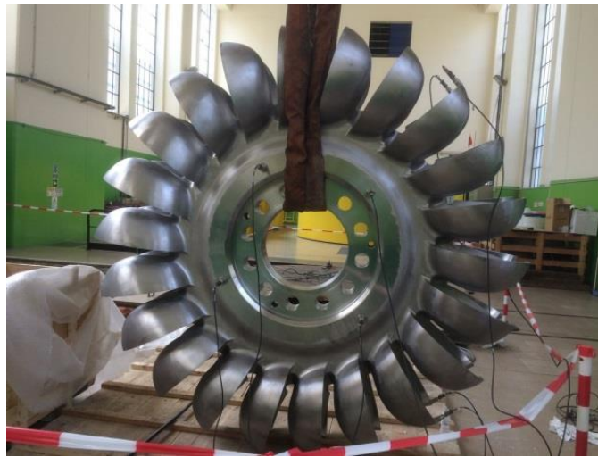
Figure 2.14. Accelerometers disposition on the hanged runner
