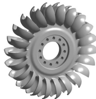
Figure 2.5. Left, view of the runner and right, CAD geometry of the runner
