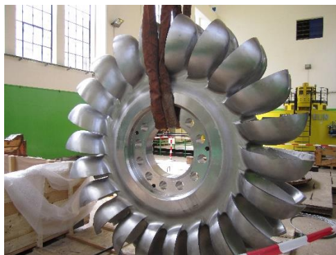
Figure 2.5. Left, view of the runner and right, CAD geometry of the runner
