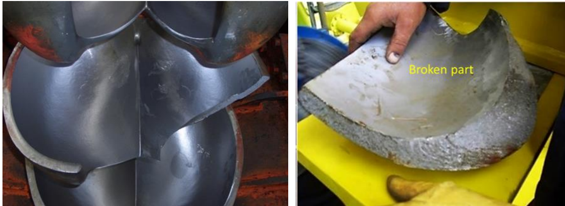
Figure 6.19. Pictures of the wheel with damage. Left, view of the broken bucket and right, detached bucket part
