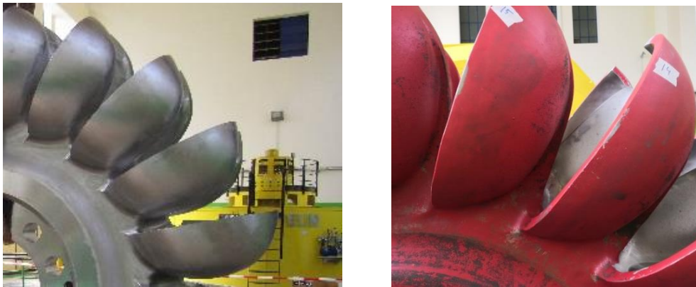
Figure 3.11. Left, runner A-1 attached to the machine and left, A-2 buckets with back supports
