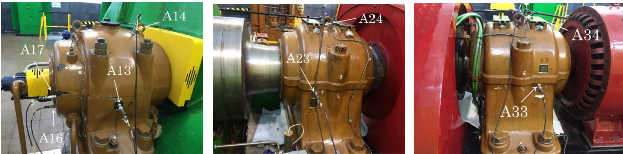
Figure 3.18. Accelerometer position on machine bearings 1 (left), 2 (middle) and 3 (right)
