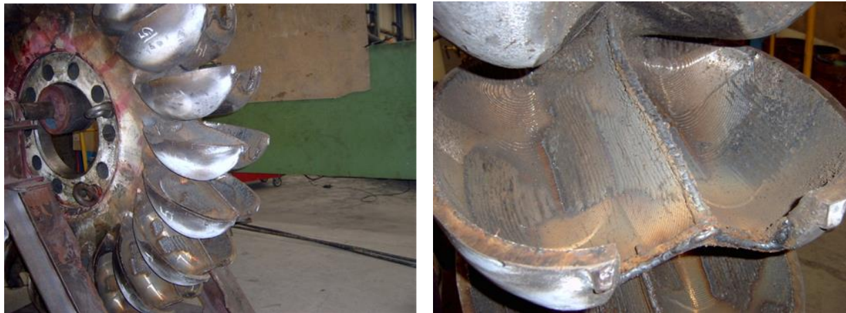
Figure 6.14. Examples of weld repair
