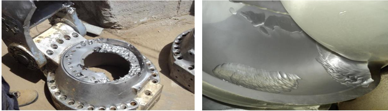
Figure 6.9. Particle erosion in Pelton turbine components
