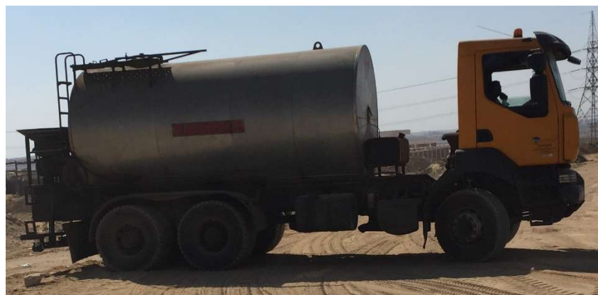
Figure 4- 9: MC & RC sprinkle machine
