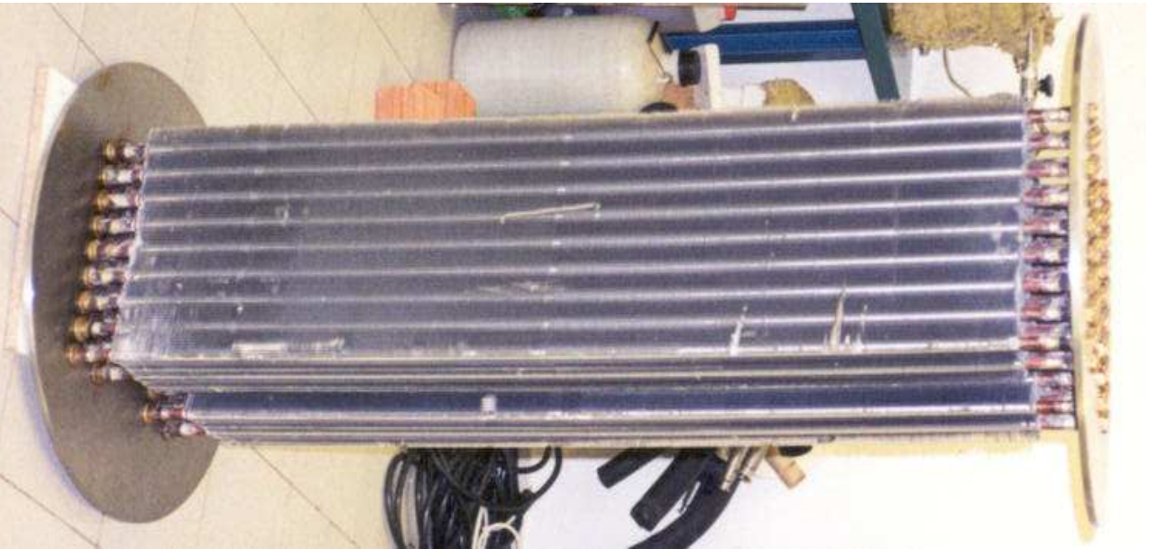
Figure 6.7: Tube-fin heat exchangers (absorber and condenser)
