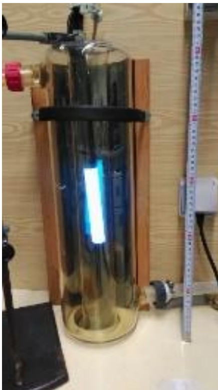
Figure 3.2. Annular photoreactor and irradiation system
