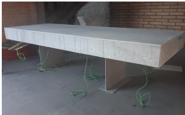
Figure 5.2. Visual aspect of the full-scale benches fabricated for the thermal characterization.
