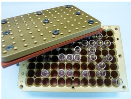
**Scheme 24.** General HTE procedure used for chiral ligand testing in synthesis of **21a** and image of HTE 96 positions reaction plate.
