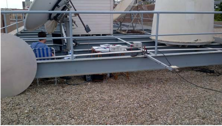
Figure 7.1: Experiment on the rooftop that lead to the discovery of the DME/TACAN interferences at L5/E5A frequency band.
