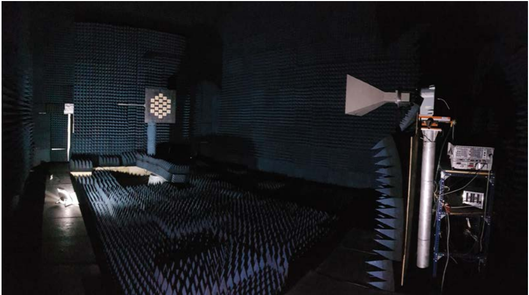
Figure 6.13: MIR down-looking array being calibrated and measured at the UPC anechoic chamber. The 19 elements MIR array is at the back left, while the transmitting reference horn antenna is at the front right. The transmitting antenna has linear polarization and can rotate around the boresight axis.
