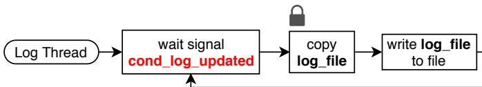
Figure 5.49: Flow diagram of the thread in charge of writing the log information to a file.
