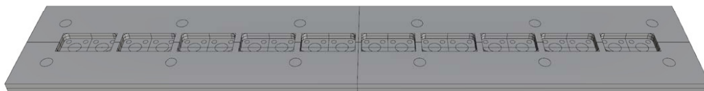
Figure D.8: 3D model of the slide used to manufacture the pieces (down). The slide measures 340x60x6 mm.
