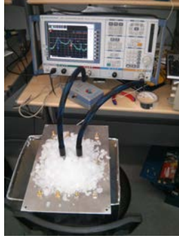
Figure 3.4: Measurement of the BEXUS antennas temperature matching response.
