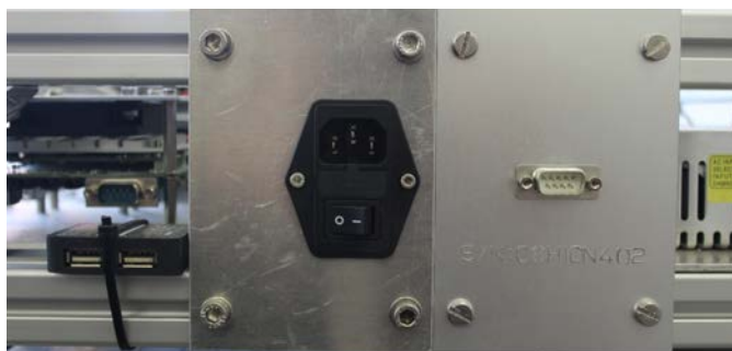
Figure H.2: From left to right, USB switch, power connector, and SPI connector.
