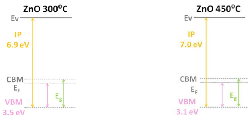
Figure 3.19 Band diagram of ZnO thin films at 300 °C (left) and 450 °C (right) determined by UPS.
