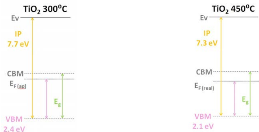
Figure 3.17 Band diagram of TiO 2 thin films at 300 °C (left) and 450 °C (right) determined by UPS and XPS.
