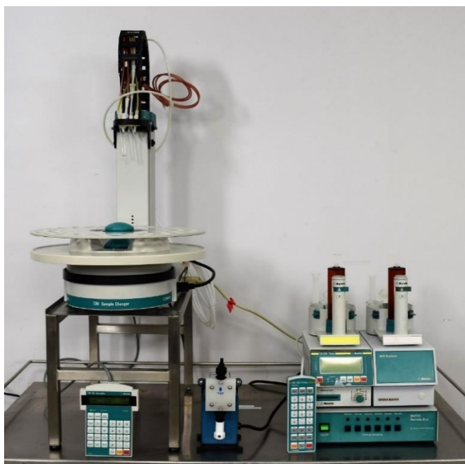
Figure 2-12 Coulometric Karl Fischer titration.
