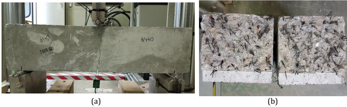
Figure 30 - Specimen after fatigue test (a) and fibre counting of cross section (b)
