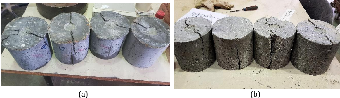
Figure 7 – Specimens subjected to Barcelona test of HPFRC (a) and SFRC (b)
