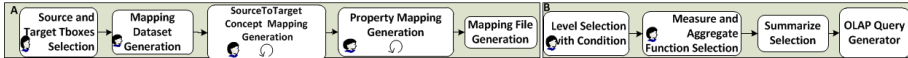
Fig. C.2: The workflows for Source2Target Mapping(A) and OLAP Query Generation (B) operation. The rectangles, user icons and curved arrows represent automatic, user-required and iterative tasks.
