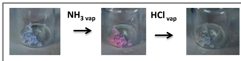
Figure 4.22: digital images of the Cyn I/DPA@HDOH microparticles in presence of \text{NH}_3 and HCl vapors.
