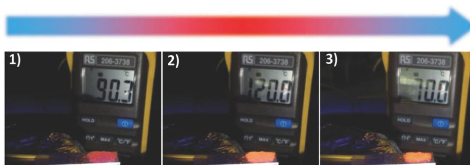
Figure 5.26: digital snapshots showing the fluorescence enhancement occurring while heating the powder from 90 to 120 °C and the fluorescence maintenance once the RhB/DA@PMMA NPs were cooled down to lower temperatures ( \lambda_{\text{exc}} = 365 \text{ nm} ).
