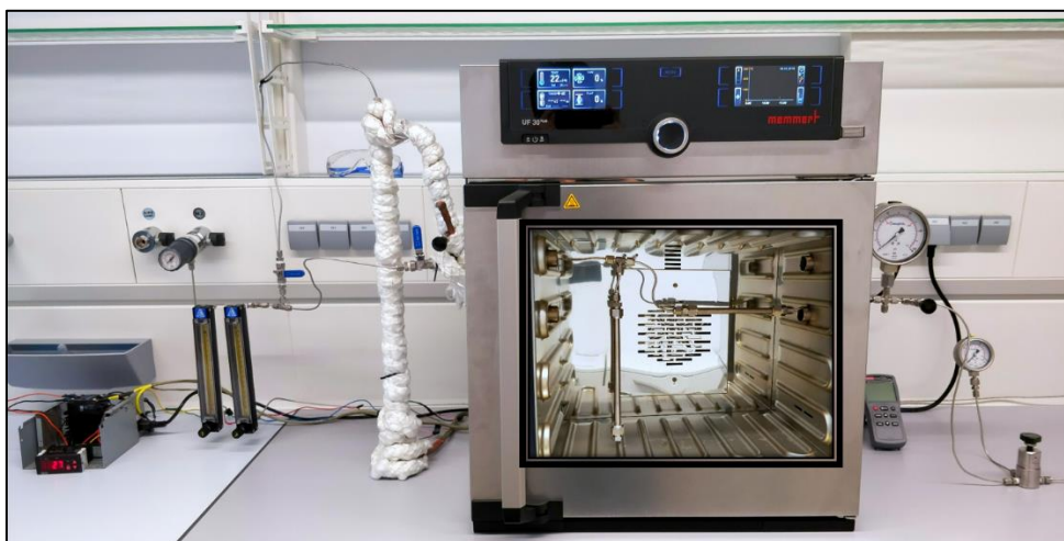
Fig. 3.2. Picture of the purpose-built steam-mediated carbonation reactor. Picture taken by K. Rausis.
