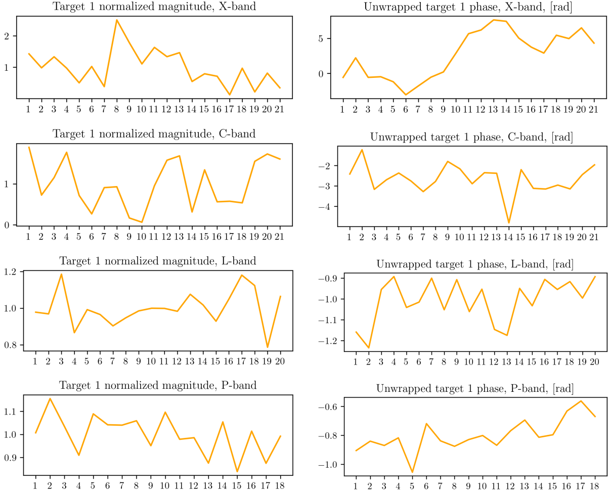
Figure 4.19: Amplitude and phase stability of the rocky area under vegetation.
