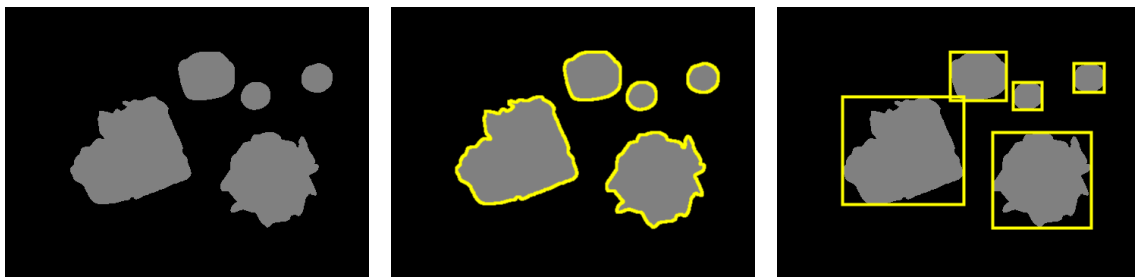
FIGURE 8.4: Food segmentation output (left to right): binary prediction by FCN, regions boundaries and food bounding boxes.
