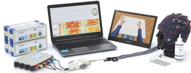
Figure 2. Components of recoveriX system
