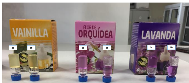
Figure S1. Gelation tests of 2c and 2b in three different commercial liquid fragrances: “Vainilla” (Vanilla, 81010750, composition: 2-metoxi- p -cresol), “Orquídea” (Orchid, 80851602, composition: linalol, 4- tert -butylcyclohexyl acetate, 3- p -cumenyl-2-methylpropionaldehide, 2-(4- tert -butylbenzyl) propionaldehide, 1,2,3,5,6,7-hexahydro-1,1,2,3,3-pentamethyl-4H-inden-4-one, 2,4-dimethylcyclohex-3-en-1-carbaldehide, damascenone, geraniol, hexyl salicilate and silcolide) and “Lavanda” (Lavender, 80961712, composition: linalol, 4- tert -butylcyclohexyl acetate, 1-(1,2,3,4,5,6,7,8-octahydro-2,3,8,8-tetramethyl-2-naphthyl)etan-1-one, cineole, 3-(4- tert -butylphenyl)propionaldehide, 3-methyl-4-(2,6,6-trimethyl-2-cyclohexen-1-yl)-3-buten-2-one, citronellol, coumarin and D -limonene).
