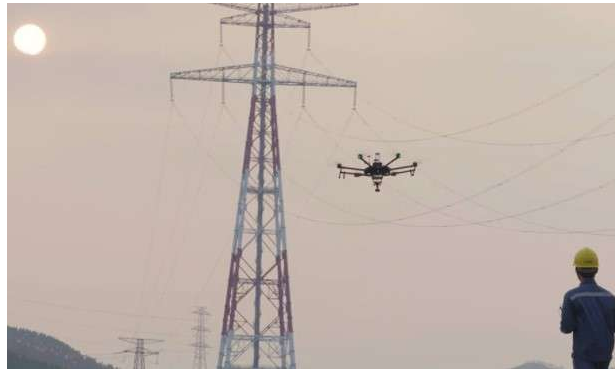
Figure 1.8: The drone operates for Electric power line patrol [WET].
