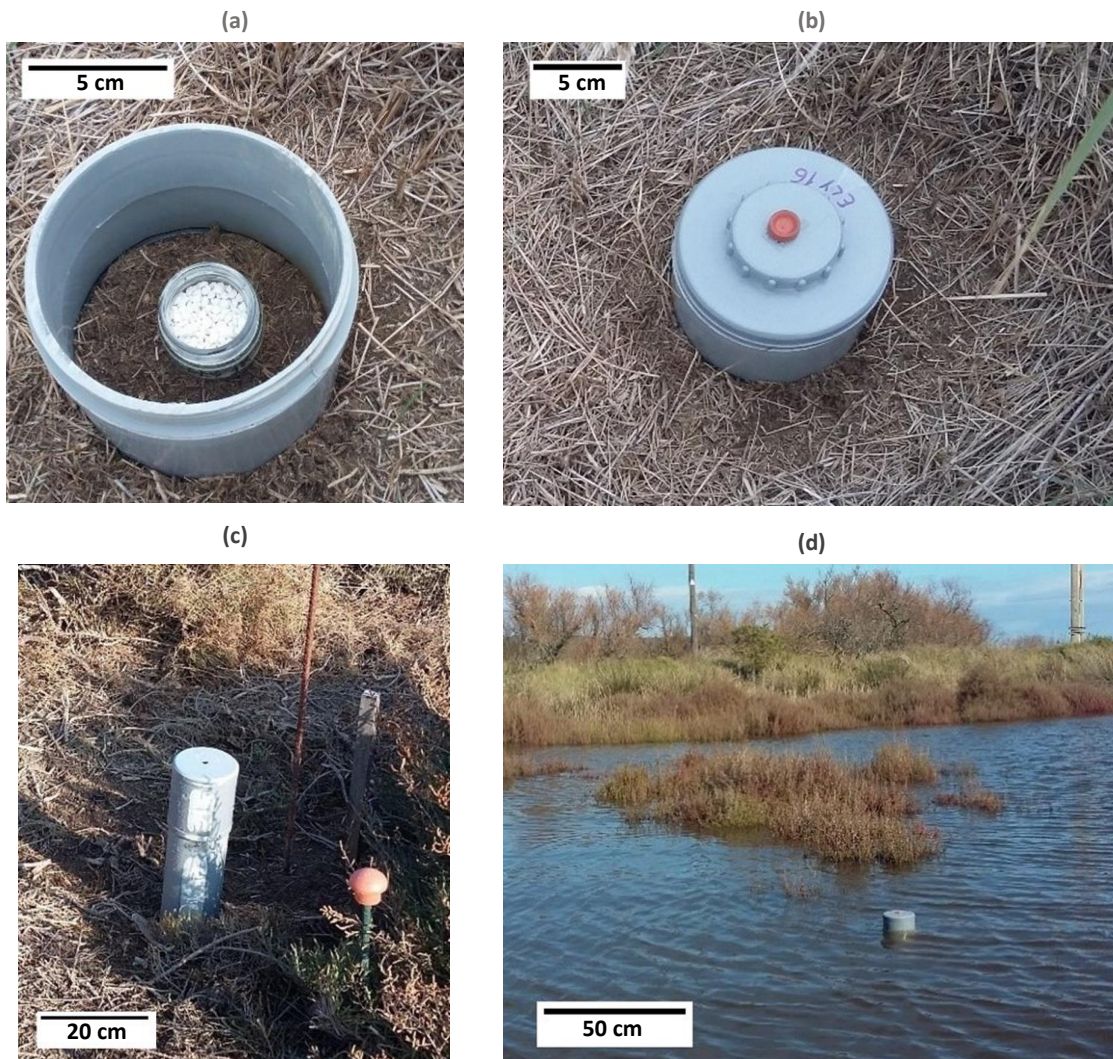
Figure 3.5. Cover boxes used to take the measurements of net \text{CO}_2 and \text{CH}_4 fluxes from soil when it was not flooded (a and b) and in the case that the soil could be flooded (c and d). When soil was not flooded, soda lime was placed inside the cover box (a) and then the cover box was hermetically closed (b).
