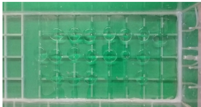
Figure 18 Lower water injection system, at the initial moment of injection.
