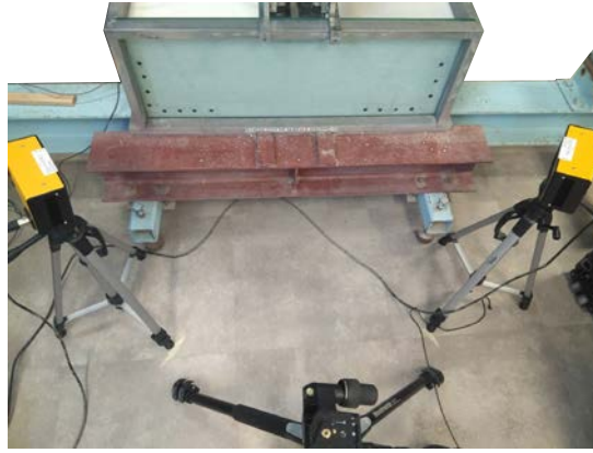
Figure 117 Light source and camera location respect to the tank.
