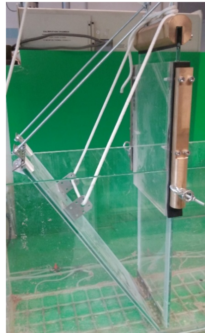
Figure 21 Guillotine with the system to fix the initial angle.
