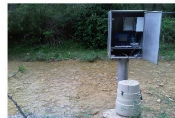
Figure 3. The Canada Hydrometric Station (Photo by David Estary). Water depth and turbidity were continuously measured by means of a pressure transmitter (Druck® 1730-PDCR) and a turbidimeter (ANALITE® NEP9350; range: 0–3000 NTU), respectively. This setting was the same in all the monitoring stations with the exception of River Fred Hydrometric Station, that it had a float with a water level sensor and a data logger.
