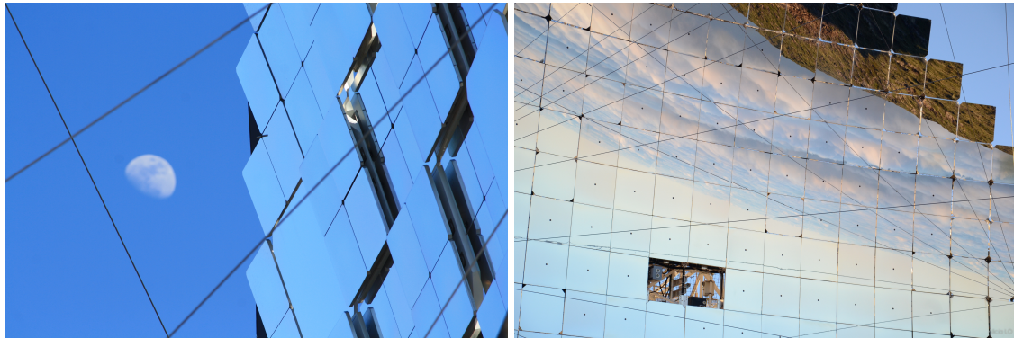
Figure 3.10 Particular of the mirror surfaces of MAGIC I (left) and MAGIC II (right).
