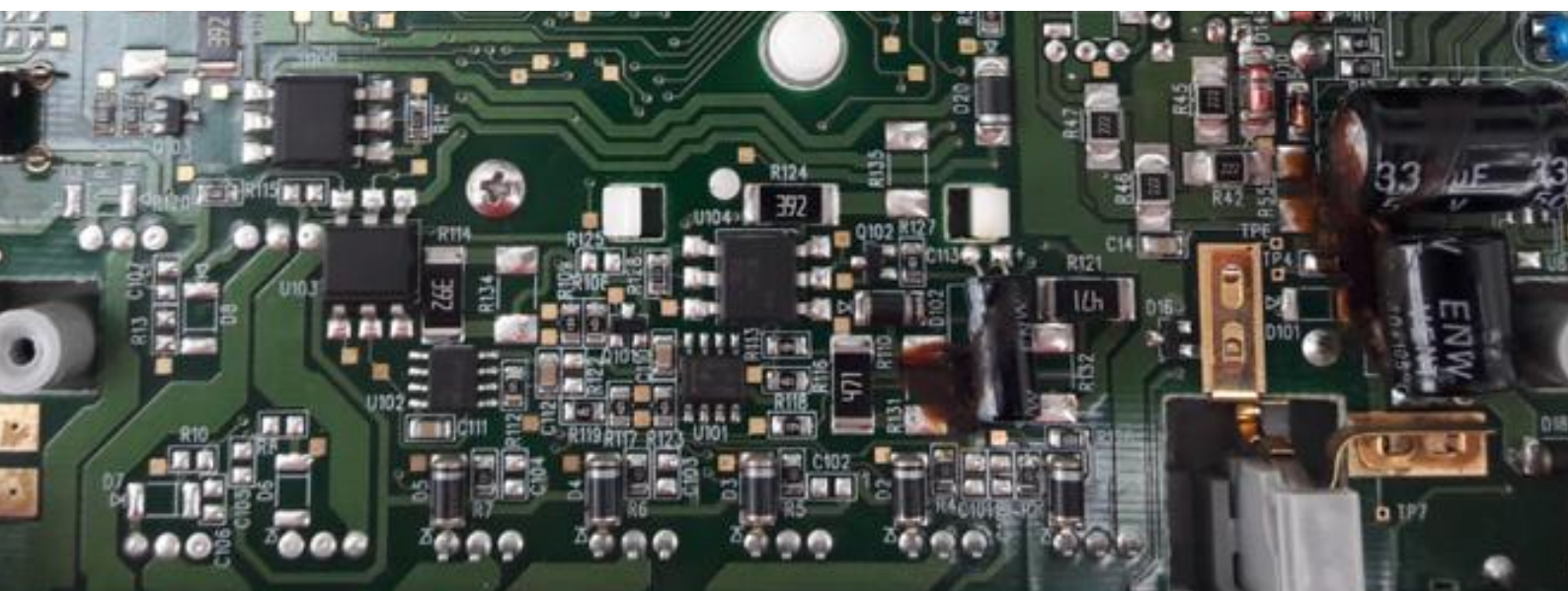
Picture: Interior of an irrigation programmer
