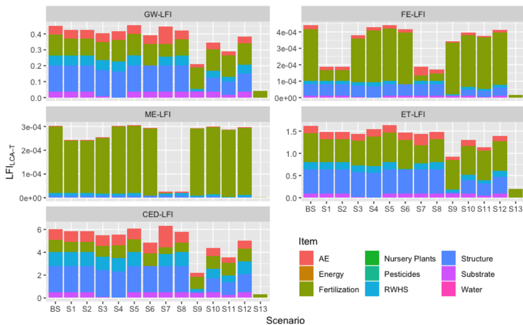
Figure 9.6 Scores for the LFI_{LCA-T} . GW: Global Warming; FE: Freshwater Eutrophication; ME: Marine Eutrophication; ET: Ecotoxicity; CED: Cumulative Energy Demand; LFI: Linear Flow Index; AE: Auxiliary Equipment; RWHS: Rainwater Harvesting System.
