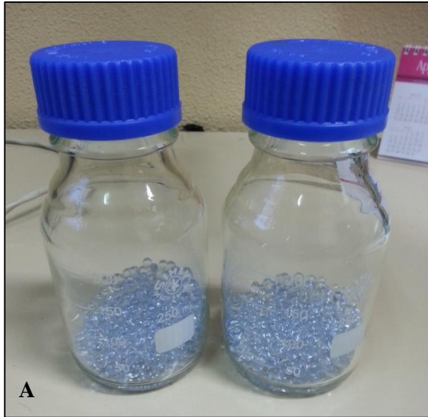
Figure 35. Glass beads (Labbox®) in 250 ml containers used for defibrinating blood (A). Containers filled with the glass beads and bovine blood (B).
