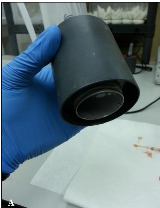
Figure 36. Parafilm® artificial membrane attached to the Hemotek© arm (A). Hemotek© arm set on top of the cardboard box with the C. obsoletus NF inside (B).
