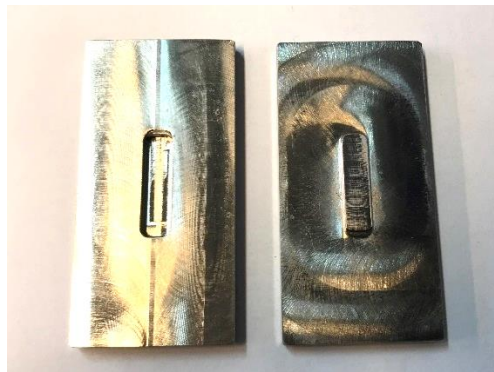
Figure 6.1 Stainless steel mold used for the specimen preparation for DMTA analysis.
