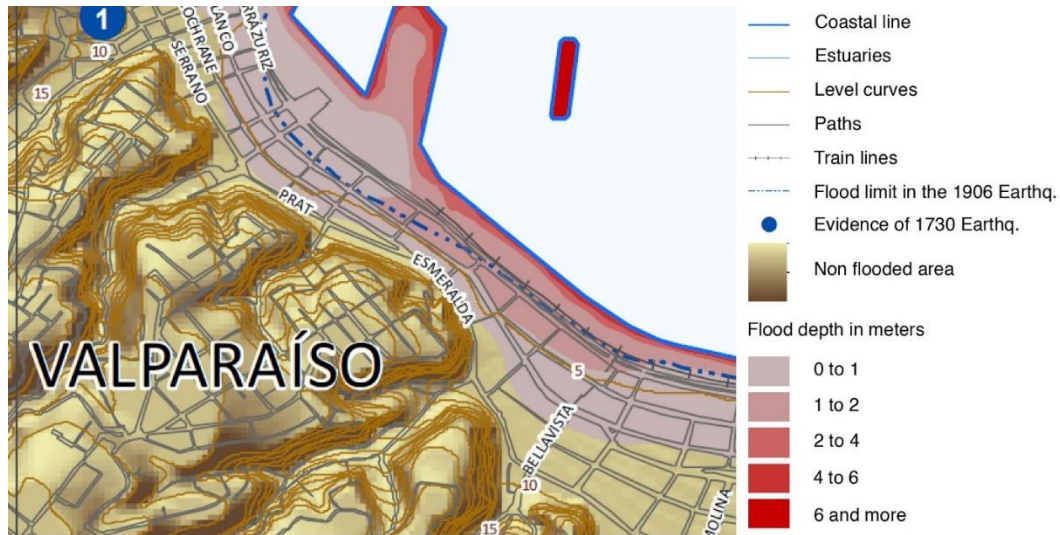
Figure 3-16. Tsunami Inundation Map of the city of Valparaíso developed by the Hydrographic and Oceanographic Service of the Chilean Navy (SHOA 2012).
