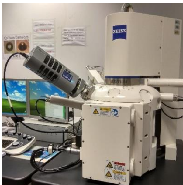
Figure 2.21: Auriga SEM at the IREC facilities.
