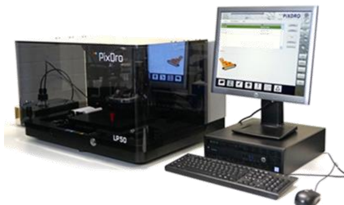
Figure 2.4: PixDro inkjet printer used at the DTU facilities (Risø campus) to print YSZ electrolytes.
