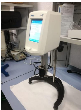
Figure 2.13: DV3T Rheometer used to measure the viscosity of the sol gel inks for inkjet printing.
