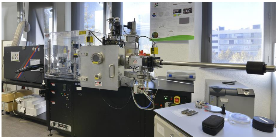
Figure 2.7: Image of the PLD-5000 from PVD® at the IREC facilities.
