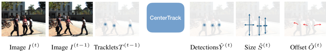
Figure 4.2: CenterTrack regression step. From two consecutive images and a heatmap corresponding to the previous detections, the centroids, widths and heights of the detections in the next time step are computed. Also, the offset between each detection from t-1 to t is outputted, and used in a posterior assignment step. Figure from [8].
