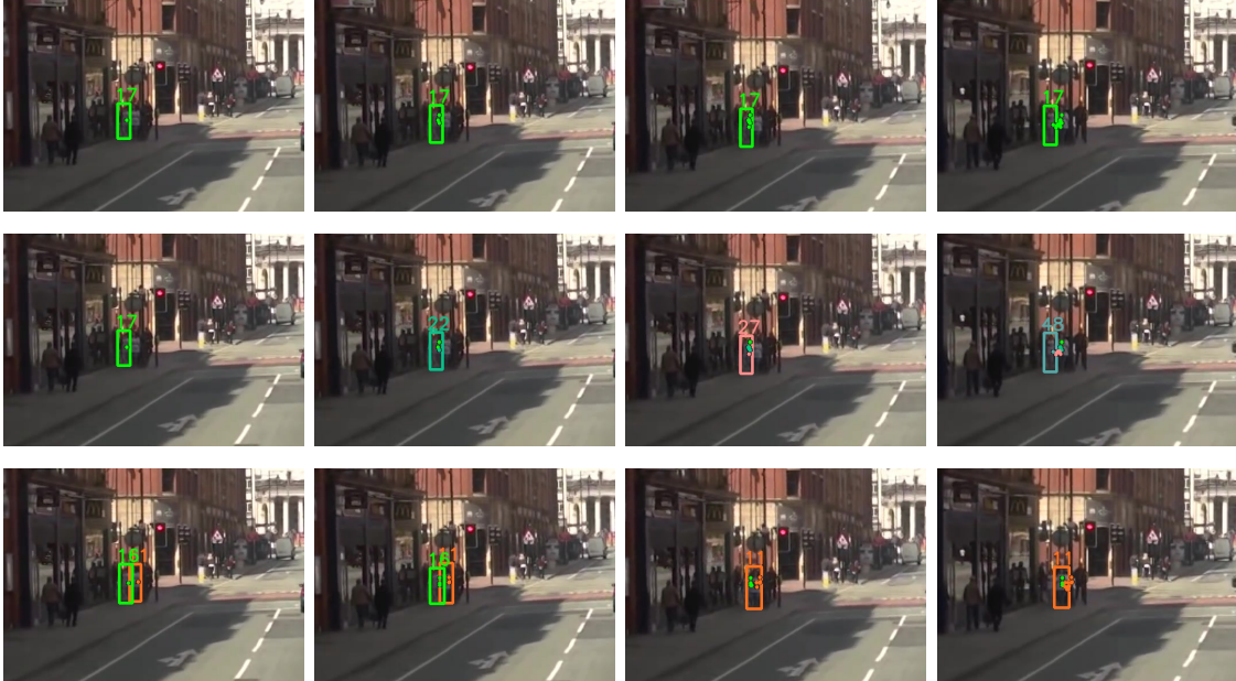
Figure 4.11: Visual example considering the AssA score between trackers. Top corresponds to the tracking of Tracktor + ReID, middle to Tracktor without ReID, and bottom corresponds to CenterTrack, where two tracks are swapped due to the association by means of the distance between centroids. Same color correspond to same track.
