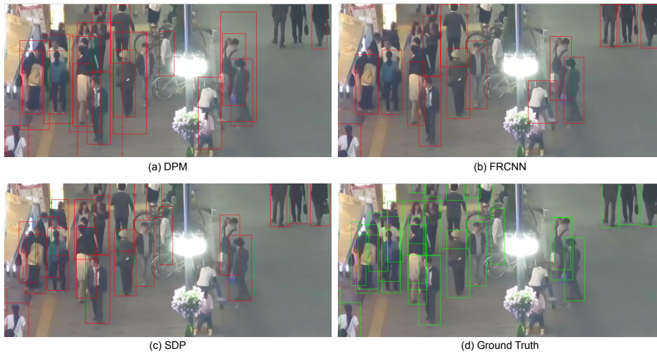
Figure 4.5: Detection samples on the three different detectors that MOTChallenge provides as public detections. The MOTChallenge testing set uses the average result from the tracking method, over the public detections from the three detectors, in order to compare to the other state of the art techniques.
