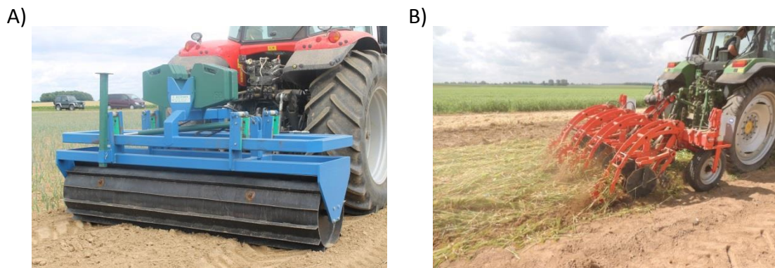
Picture 1. Machinery used for NT-RC management in the Walloon Agricultural Research Center (BE-CRA-W) trial. A - Roller crimper; B - In-line tiller.
