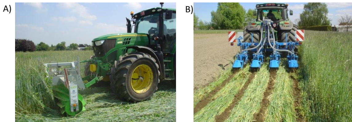
Picture 5. Machinery used for NT-RC management at the INAGRO (BE-INAGRO) organic farm station. A - Roller crimper; B - In-line tiller.
