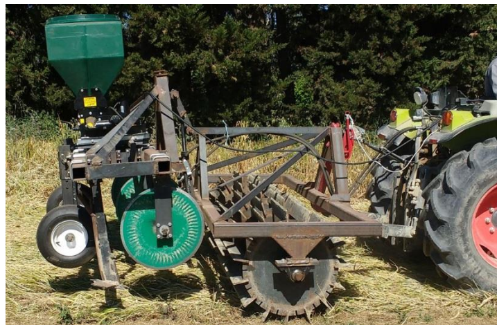
Picture 14. Machinery used for NT-RC management at the experimental organic research centre of the Groupe de Recherche en Agriculture Biologique (GRAB) in Avignon (FR). A tractor equipped with a roller crimper and an in-line tiller.
