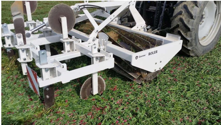
Picture 18 Machinery used for NT-RC management in the trial established at the University of Maribor (Pivola), Faculty of Agriculture and Life Sciences (UM), Slovenia (SI). A tractor equipped with a roller crimper and in-line tiller.
