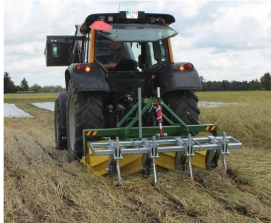
Picture 9. Machinery used for NT-RC management in the organic research field at Jõgeva in eastern Estonia (EE). A tractor equipped with a roller crimper and an in-line tiller.
