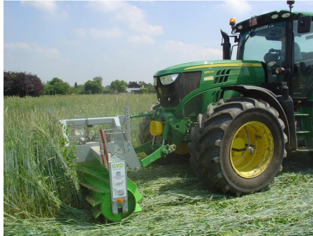
Picture 3. The roller crimper flattening the ASC in the Research Institute for Agriculture, Fisheries and Food (BE-ILVO) trial.
