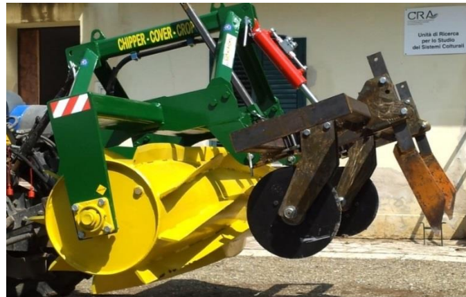
Picture 16. Machinery used for NT-RC management at the Experimental Farm of Metaponto belonging to the Consiglio per la Ricerca in Agricoltura e l'Analisi dell'Economia Agraria (CREA) in southern Italy (IT). A tractor equipped with a roller crimper and in-line tiller.
