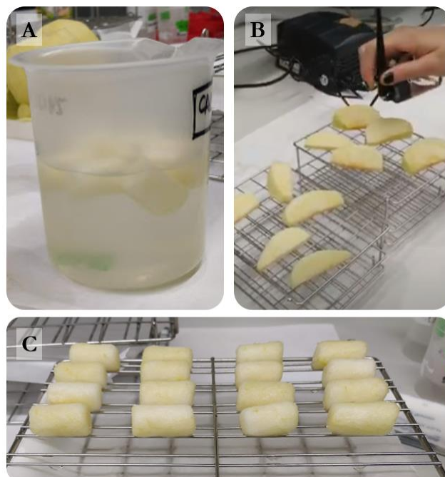
Figure 66. (A) Immersion of apple slices in FA solution, (B) spraying FA slices with FA solution, and (C) drying of melon disks after their inoculation with Salmonella enterica BAA-707 for FA trials.
