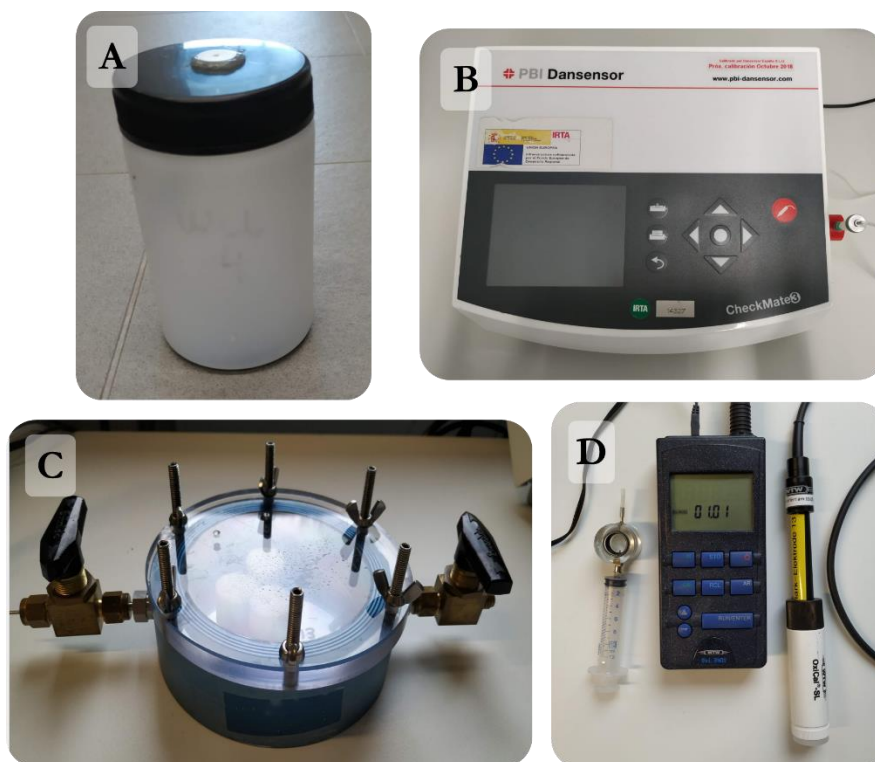
Figure 71. Respiration rate measurement equipment. (A) is CheckMate Dansensor, measurement of O_2 and CO_2 , (B) the hermetic pot with a septum, (C) is Oxi 34i Meter for measuring O_2 , and (D) hermetic cell with two valves for gas inlet and outlet.
