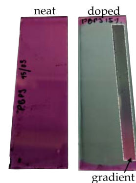
Figure 4.7: Neat and doped films of PBTTT. Inset is a section of a PBTTT film with a dopant gradient.
