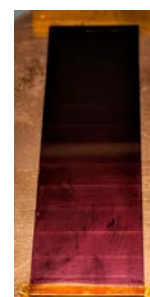
Figure 4.3: Film of RR-P 3 HT deposited using the blade coating technique
