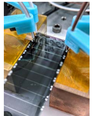
Figure 4.15: Picture of the two-probe configuration setup.
