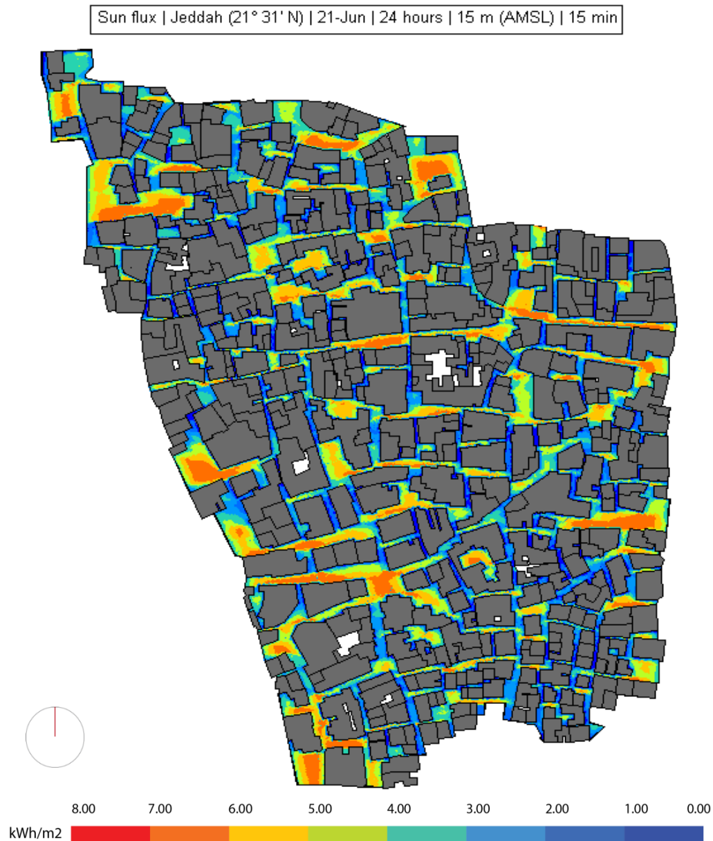
Figure 1.31. AlBalad (the old layout) summer, 21 st of June, solar flux. Source: Heliodon software.
