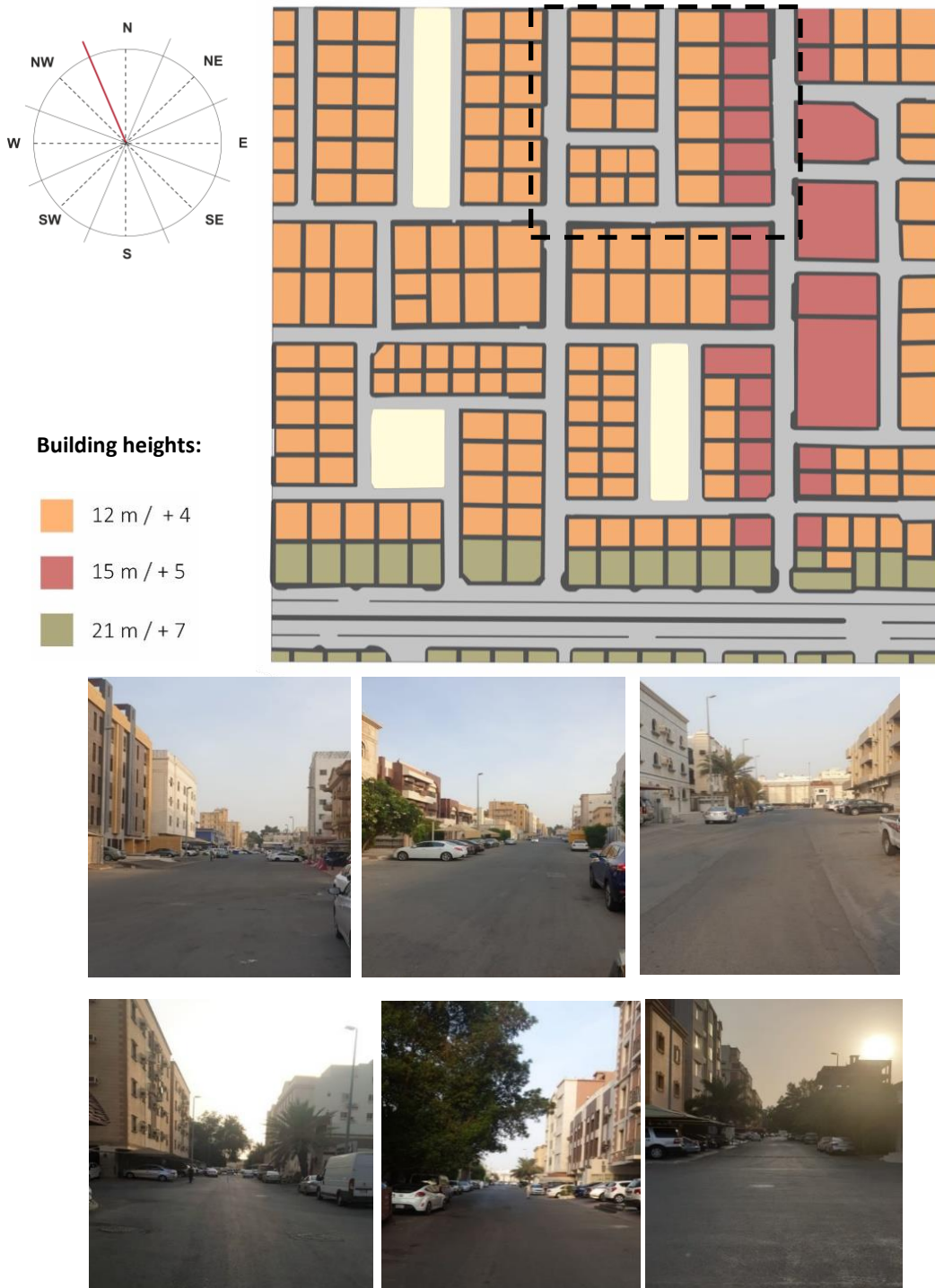
Figure 5.20. Case A: the existing urban layout (above), showing the building heights and the applied proposal represented in the dotted square. The pictures at the bottom show the actual streets of the layout.
