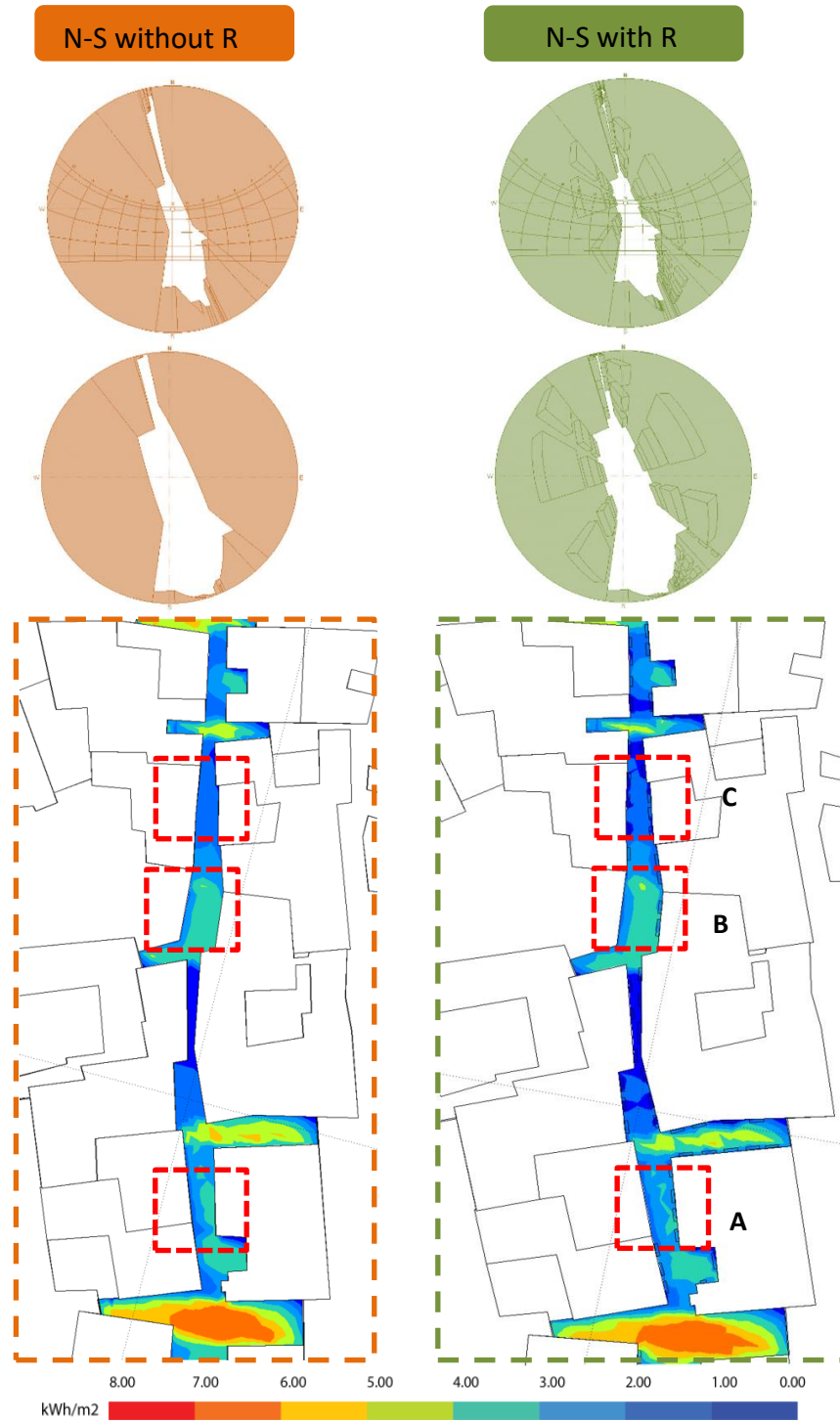
Figure 5.4. The amount of solar flux in an N-S street: comparison of the street with and without the Rawashin. The circles on the top indicate the street projection (stereograph and orthograph) with and without the Rawashin, whereas the bottom pictures show the solar flux without (left) or with Rawashin (right) highlighting the three different Points A, B, and C.
