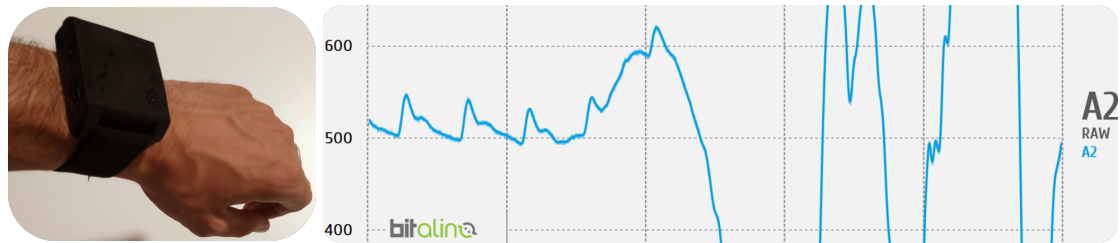
Figure 3.2: Study of blood volume pulse (BVP) noise in a custom-made wrist PPG sensor
