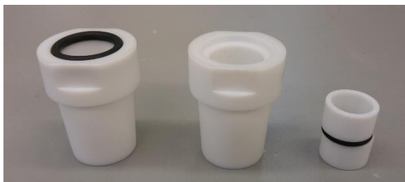
Figure 2.3. Teflon adaptors to use Schlenk tubes in the photoreactor.
