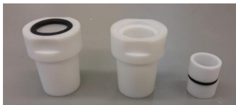
Figure 3.8. Teflon adaptors to use Schlenk tubes in the photoreactor.
