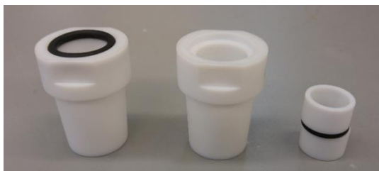
Figure 4.6. Teflon adaptors to use Schlenk tubes in the photoreactor.
