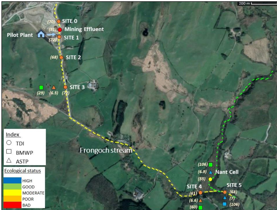
Figure 4.7: Ecological status of Frongoch stream based on diatom and macroinvertebrates indexes along the stream. TDI: Trophic Diatom Index, IB: Biological Diatom Index, BMWP: Biological Monitoring Working Party, ASPT: Average Score Per Taxon. The numbers indicate the value of each index and the colors the category of water quality.
