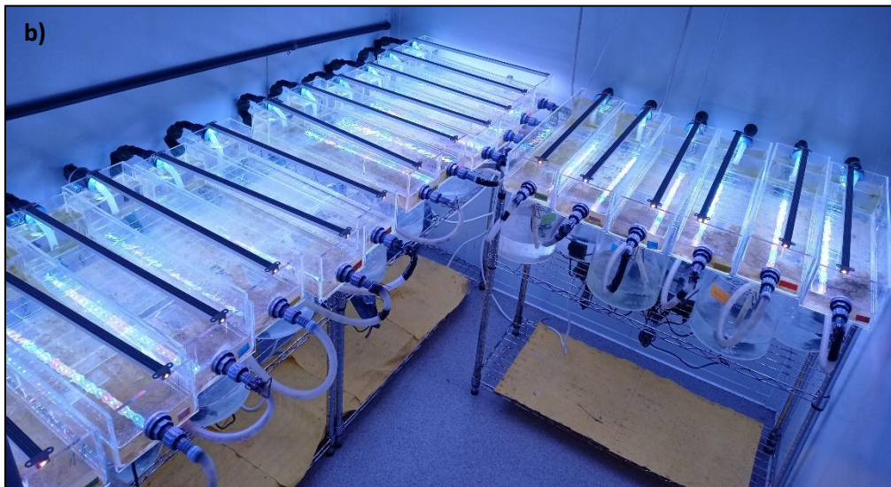
Figure 3.3: Artificial streams: a) scheme of the artificial streams. b) artificial streams placed in the chamber under controlled conditions.
