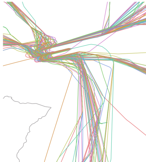
Figure V-2: Arrival traffic on September 14th, 2018 in Frankfurt airport obtained from OpenSky ( The OpenSky Network, 2019 ) automatic dependent surveillance-broadcast (ADS-B) trajectories
