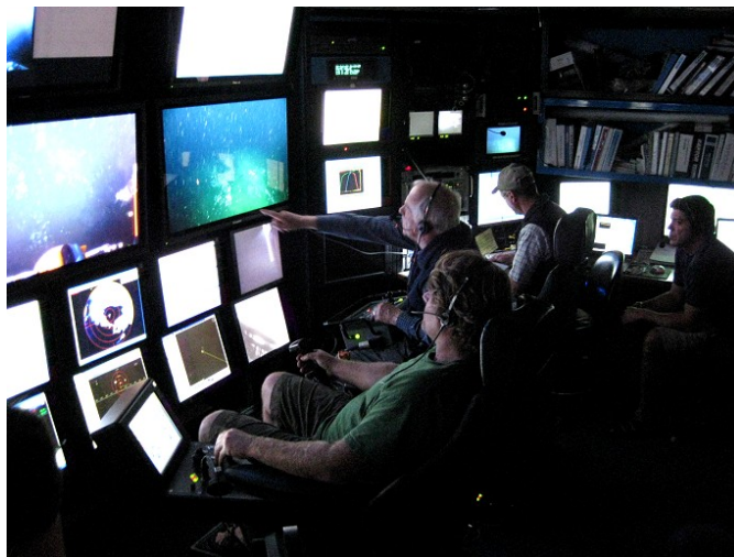
Fig. 5.4 A typical ROV Control Room (courtesy of Monterey Bay Aquarium Research Institute).
