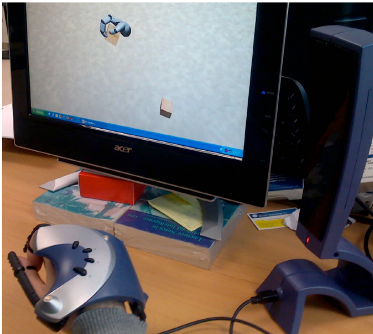
Fig. 5.2 Detail of the P5 data glove during a simple test: ‘grasp a virtual cube’.
