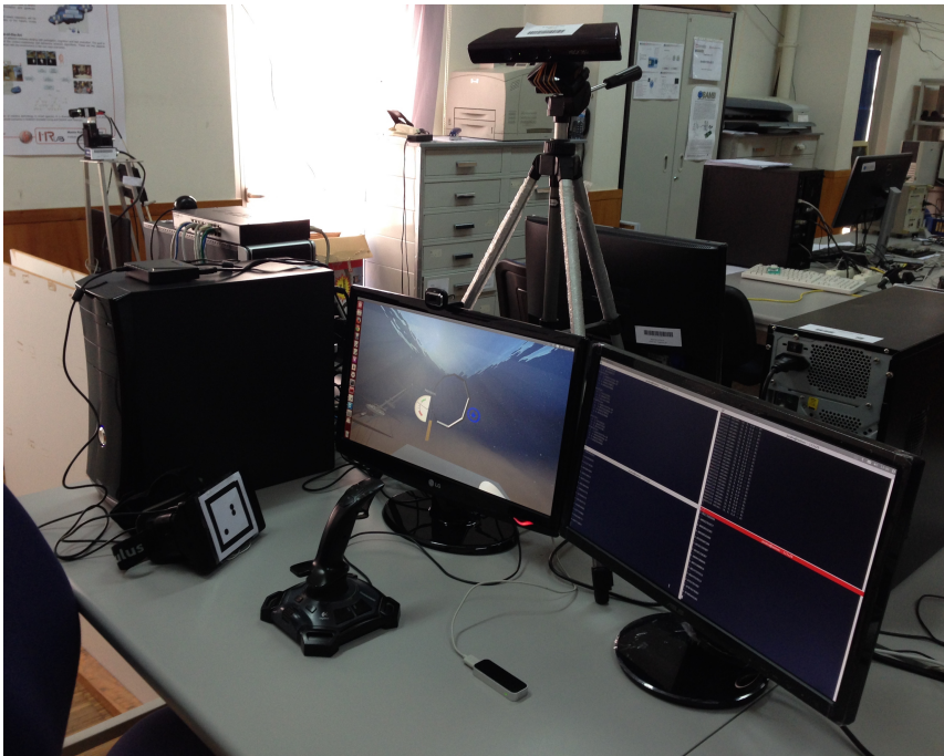
Fig. 5.14 The Microsoft Kinect™ should be place behind the monitors in order to keep the user inside the workspace.
