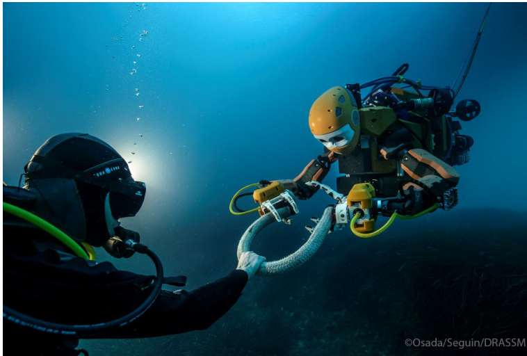
Fig. 2.4 New underwater robots: Ocean One, a bi-manual underwater humanoid robot.
