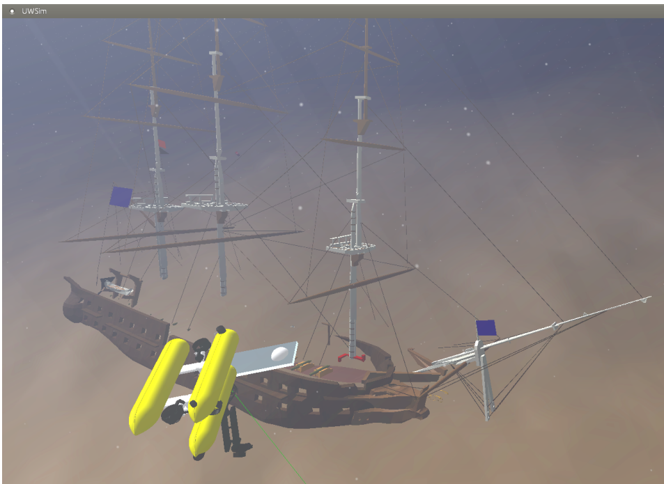
Fig. 6.2 Scene from the UWSim. The robot navigates to a position defined by the user. The shipwreck represents an unavoidable obstacle, because the ropes are hardly detectable by the robot sensors.
